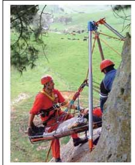
AZ Vortex Multipod used as an easel A frame during a 2005 Ropes That Rescue training in New Zealand.
